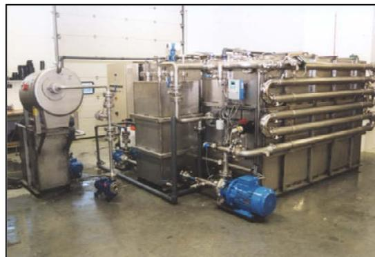
Eventually, the idea came to re-use the effluent for flushing toilets to avoid seawater in the system. Beginning of 2002 rebuilding of the installation was started on board. Tests in April showed how good the choice of recirculation of the effluent had been. Results of the purified water were good and the process was stable.
